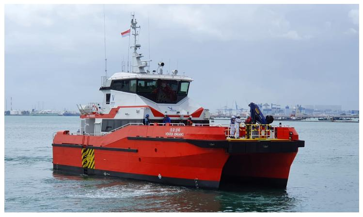
BV: I HULL MACH Wind farms service ship - S0 - Sea Area 2 CR: CR100+ Aluminium Alloy Hull, Work Boat, LSC, Greater Coastal Service, CMS+
