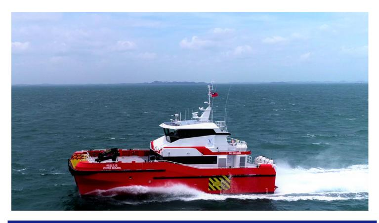
BV: I HULL MACH Wind farms service ship - S0 - Sea Area 2 CR: CR100+ Aluminium Alloy Hull, Work Boat, LSC, Greater Coastal Service , CMS+
