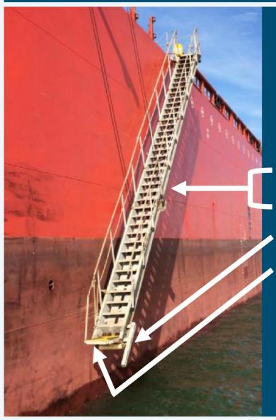
When vessel is underway, accommodation ladder shall not be used unless it is deemed necessary.
