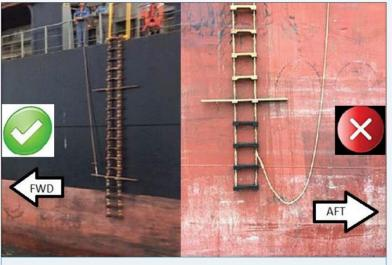
Retrieval line if used, should be fastened at or above the last spreader and should lead forward.
