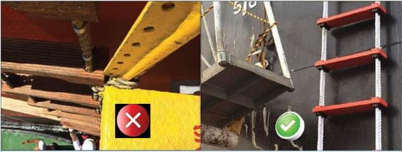
Horizontal distance between pilot ladder and lower platform should be between 0.1 and 0.2 m. [2] [8]
